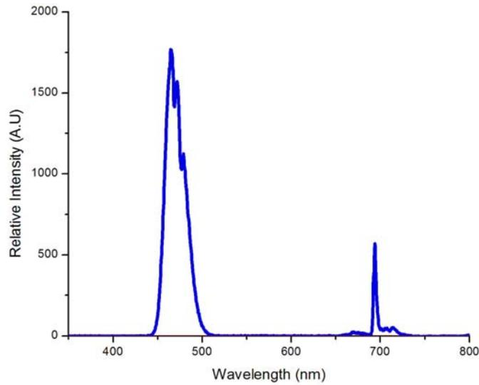
**Figure 9 Spectrum from super Blue LED and Ruby**
