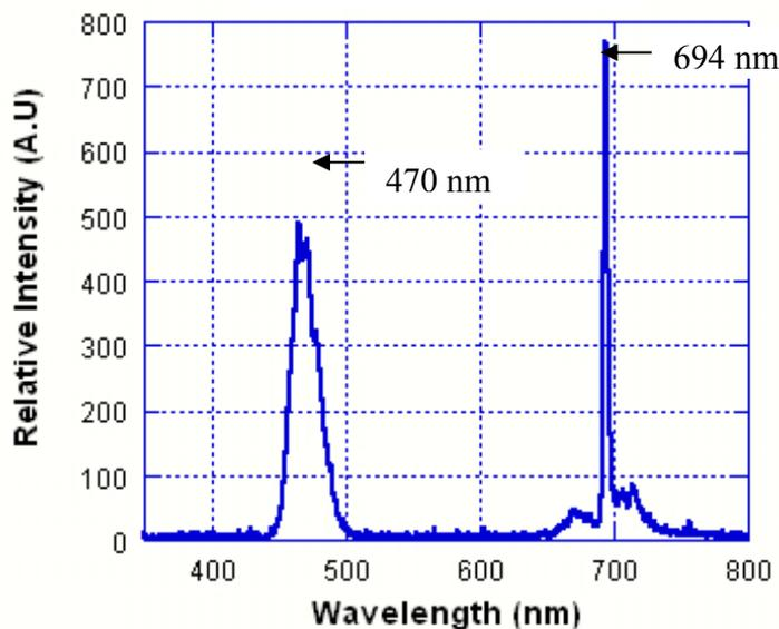
Figure 5 Spectrum of Commercial Blue LED with Ruby [13]
