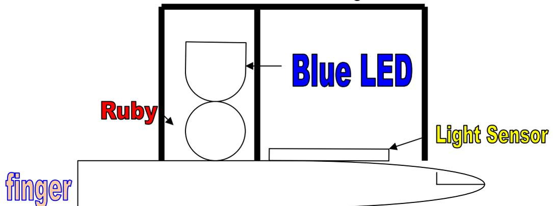
Figure 12. Diagram for reflectance oximetry.
