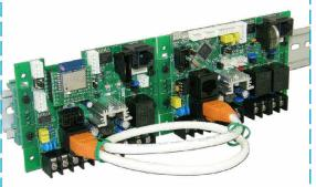
It illustrates how to connect ET-MEGA32U4-RS485 with ET-ESP8266-RS485.
