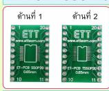
It is PCB CONVER for IC 20PIN SSOP and 20PIN TSSOP with 0.65mm. PITCH to convert to be 20PIN DIP TYPE (15.24mm, width). PCB SIZE is 1.8 x 2.5 cm.
