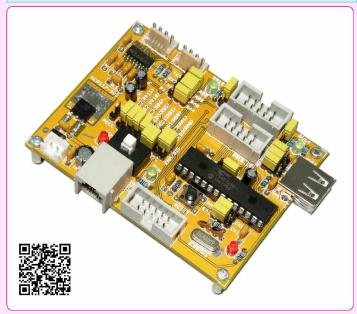
This is the latest ETT Board in the series of PIC32MX of MICROCHIP; it uses 32 BIT MCU No.PIC32MX250F128B 28- on board.
