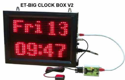
• An example illustrates how to connect ET-BIG CLOCK BOX V2 to ET-GPS-RS485.
