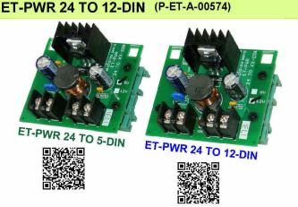
This POWER SUPPLY is provided with fastener to attach with RAIL DIN 35mm. It is STEP-DOWN VOLTAGE REGULATOR OUTPUT 3A that uses IC No.LM2576-XX. There are 2 sizes of OUTPUT as follows;
