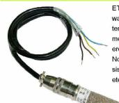
ET-SHT10 WATER PROOF SENSOR is waterproof and durable Sensor to measure temperature and humidity; it can accurately measure humidity in the air and soil (not covered with water) well. It uses IC SENSOR No.SHT10 that is contained in the water-resistant box. The SENSOR is 79mm; Diameter is 14.50mm; and Cable is 50 CM long.
