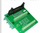
HEADER CONNECTOR 2.54mm 30 PIN is converted to CONNECTOR TER-MINAL SCREW PITCH 3.50mm 30 PIN with 2 of RAIL DIN 35 mm. and PCB SIZE is  $7.89 \times 7.40$  cm.
