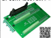
HEADER CONNECTOR 2.54mm 34 PIN is converted to CONNECTOR TERMINAL SCREW PITCH 3.50mm 34 PIN with 2 of RAIL DIN 35
