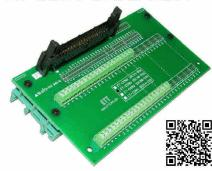
HEADER CONNECTOR 2.54mm 40 PIN is converted to CONNECTOR TERMINAL SCREW PITCH 3.50mm 40 PIN with 2 of RAIL DIN 35
