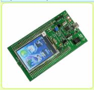
This 32 BIT MICROCONTROLLER Development kit is in the series of STM32F429/439 from ST; this inexpensive Board provides ST-LINK V2 on board that is ready to develop. Board is divided into 2 parts as follows;
