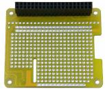
It illustrates how to connect ET-PROTO HAT, it solders 2 x 20 STACKABLE 25.5 mm. onto Board RASPBERY Pl.
