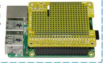
This ET-PROTO HAT or multi-purposed PCB as HAT (HARDWARE ATACHED ON TOP) is specifically designed for use with Board RASPBERRY PI that has Connector 40 PIN such as PASPBERRY PI MODEL A+, RASPBERRY PI MODEL B+, RASPBERRY PI2 MODEL B; it is suitable to make prototype boards by connecting with RASPBERRY PI via Connector 40P conveniently. SPECIFICATIONS of Board ET-PROTO HAT
