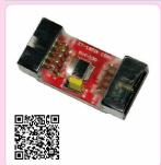
This mini board with 2 of Connector 10PIN ET BUS I/O is designed for use with PAIR Cable 10PIN conveniently. It is connected with Signal LOGIC between 5V devices with 3.3V devices by using IC 74LCX245 to be intermediate. It can setup JUMPER for all 8BIT. It can send data from 5V side to 3.3V side or from 3.3V side to 5V side by Circuit REGULATOR 3.3V. It is suitable for connecting Board MCU that is 3.3V I/O with 5V I/O Board.
