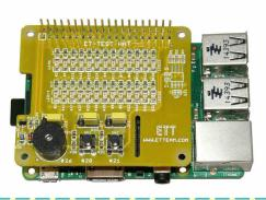
Board ET-TEST HAT is specifically designed to test I/O PORT of Board RASP-BERRY PI; it is used to test the operation or write sample program to show on LED Display or BUZZER on this board.
