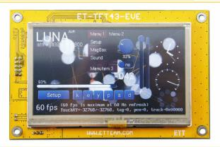
ET-TFT43-EVE is Board TFT LCD 4.3 Inch that works with CHIP FT800, it is easy to use TFT LCD. It is SPI Interface and supports both 3.3V I/O and 5V I/O. It can interface with both 3.3V MCU and 5V MCU, but, the Power Supply of board must be 5V only.
