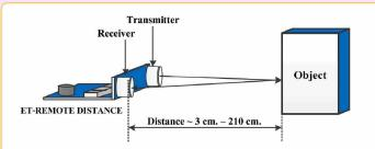
It illustrates how to measure distance of MODULE ET-REMOTE DISTANCE.
