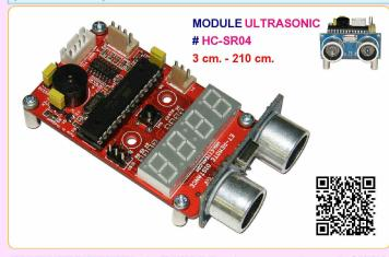
ET-REMOTE DISTANCE is the MODULE Board to measure distance by ULTRA-SONIC Wave "HC-SR04". It sends out Signal ULTRASONIC Wave and this ULTRASONIC Wave is reflected and sent back to CONTROLLER after touched any object; this Controller reads and converts the received signal into the value of distance (centimeter); and finally, it shows the result through LED-7 SEGMENT and PORT RS232.
