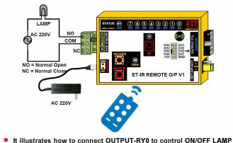
For type of REMOTE IR, it can be general REMOTE Control of TV; it has to setup the Remote(LEARNING) with the Box ET-IR REMOTE 0/P V1 first to save the setup buttons for CONTROL. These REMOTE Controls are tested and warranted they are available; NEC, SONY, RC5(PHILIP), RC6, DISH, SHARP, PANASONIC, JVC, SANYO and etc.
