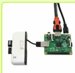
Because the Raspberry Pi MODEL A+ has no any PORT LAN, it has to use USB WIFI to connect internet for loading data as shown in the picture. In the picture, it illustrates how to connect USB WIFI with Receiver device to receive signal from keyboard and mouse through USB HUB because MODEL A+ has only one PORT USB Channel.
