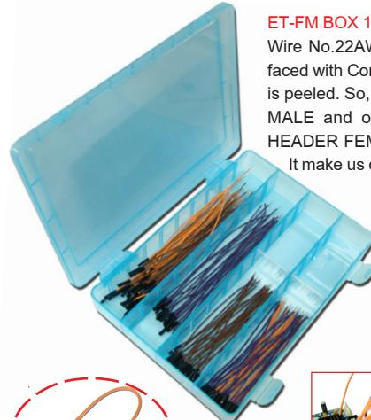
**ET-FM BOX 120** which is a kind of single Jumper Wire No.22AWG is stiff type. One side is interfaced with Connector Female and other one side is peeled. So, it can be interfaced with HEDAER MALE and other one side is interfaced with HEADER FEMALE or PROJECT BOARD.
