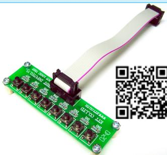
It is experimental board for test Input of ETT's Ports as 10 PIN ET BUS I/O or 10 PIN I2C IN/OUT such as in board CP-AVR V4, CP-JR908GP32 V2, CP-PIC V4, CP-JR51AC2 V2, CP-BS2P40, CP-JRBS2P40, and etc. There's 8 channel Mini Switch SW Input.
