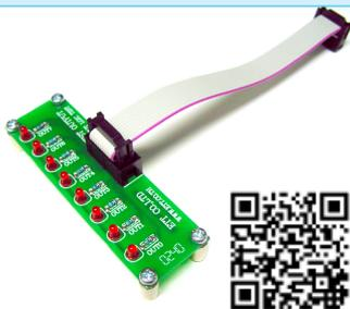
It is experimental board for test Output of ETT's Ports as 10 PIN ET BUS I/O or 10 PIN I2C IN/OUT such as CP-AVR V4, CP-JR908GP32 V2, CP-PIC V4, CP-JR51AC2 V2, CP-BS2P40, CP-JRBS2P40 and etc. It uses 8-CH.LED for test and display Output.
