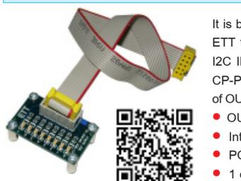
It is board to test OUTPUT of PORTs on board from ETT that is Connector 10PIN ET BUS I/O or 10PIN I2C IN/OUT such as Board ET-BASE, CP-AVR V4, CP-PIC V4. It uses LED to show the operating status of OUTPUT...
