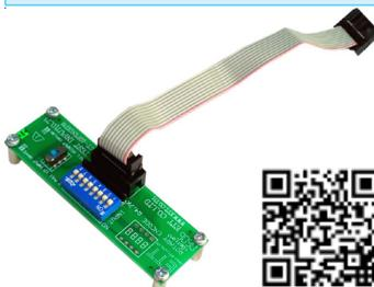
It is experimental board for test Input of ETT's Ports as 10 PIN ADC I/O such as CP-AVR V4, CP-JR908GP32 V2, CP-PIC V4, CP-JR51AC2 V2 and etc. with 8-CH.DIP SW.
