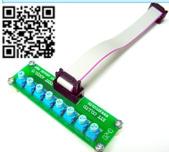
It is experimental board for test A-TO-D and D-TO-A Input of ETT's Ports as 10 PIN ADC I/O such as CP-AVR V4, CP-JR908GP32 V2, CP-PIC V4, CP-JR51AC2 V2 and etc.
