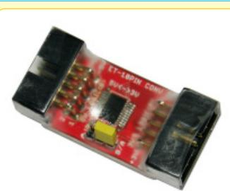
It is small board with 2 Connector 10PIN ET BUS I/O; it can be interfaced with 10PIN PAIR Cable conveniently. It is used to interface Circuit Signal LOGIC between 5V device and 3.3V device by using IC 74LX254 to be intermediate. It can set all 8BIT jumper. It can send data from 5V to 3.3V or from 3.3V to 5V, including Circuit 3.3V REGULATOR. It is suitable for Board MCU 3.3V I/O that is interfaced with Board 5V I/O.
