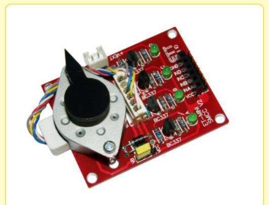
It is MINI Board Set to test STEPPING MOTOR that has been improved to interface with power supply to drive external STEPPING MOTOR; moreover, there is a particular Power Supply to drive Stepping Motor. It uses IC No.MC34063 and 4-Coil STEPPING MOTOR. It uses 4 of TR BC337 with LED to display the operating status and indicator to show directional rotation of Connector PIN HEADER 6 PIN.
