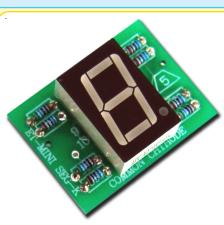
It is circuit of 7-Segment Red 1 Digit with R circuit connect with 7-Segment INPUT 10 PIN FEMALE and be able to connect with PORT I/O 10 PIN ETT directly.
