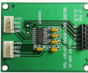
It is experiment or connect with RS232 circuit. Be able to use Power Supply VCC 3V to 5VDC and be able to connect RS232 2 channel 4 PIN ETT PORT HEADER MALE 6 PIN AND FEMALE 6 PIN. Use IC DRIVER NO.ADM3232 OR other replaceable number.
