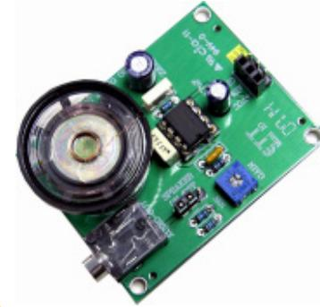
It is a mini amplifier with mini speaker on Board and STEREO JACK to connect with headphone or external amplifier set.
