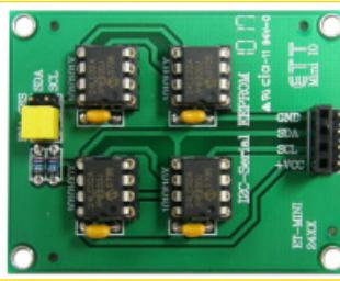
It is experiment of I2C by using 2 KBYTE IC EEPROM NO.24LC16 4 CHANNEL and be able to use in different point of I2C PORT HEADER MALE 4 PIN and FEMALE 4 PIN.
