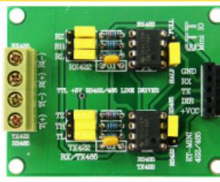
It is experiment or connect with RS422/485 circuit by using IC 75176 x 2 and connecting in RS422 or RS485 Type with Jumper. Be able to set PORT HEADER MALE 5 PIN and FEMALE 5 PIN.
