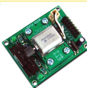
It is experiment of DC MOTOR Circuit with OPTO INPUT SENSOR 2 channel. It uses to test direction of rotation and speed of DC MOTOR with detected fan blade. It uses IC NO.L293D for DC MOTOR and PORT INPUT 7 PIN MALE/FEMALE.
