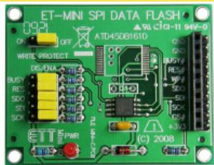
It is a Board of 2MBYTE FLASH Memory by using IC No.AT45DB16 from ATMEL, so it can be applied for storing data or DATA LOGGER.
