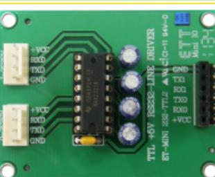
It is experiment or connect between RS232 with VCC 5VDC / 2 channel RS232 4 PIN ETT PORT HEADER MALE 6 PIN and FEMALE 6 PIN uses IC DRIVER NO.MAX232.
