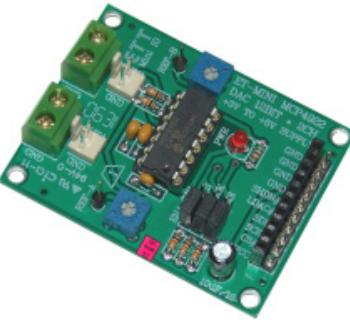
It is one of ET-MINI BOARD that is Circuit D TO A 12 BIT 2 CH and use IC No.MCP4922 from MICROCHIP.
