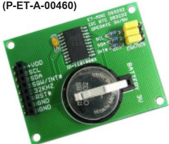
It is Circuit RTC in the format of I2C BUS that has CRYSTAL OSC inside; so, it is highly accurate to run other than RTC versions. It uses RTC No.DS3232; runs by 3V-5V, has 236 BYTE Internal RAM; with BATTERY 3V for Backup. It uses Connector 8PIN INPUT MALE and FEMALE.
