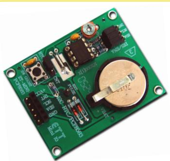
It is circuit of I<sup>2</sup>C BUS in RTC Type No.PCF8583 from PHILIPS CO, LTD.with Battery 3 V for Backup data in RTC and TACT SW. It makes RTC as Counter and Port INPUT signal as 5 PIN MALE/FEMALE.
