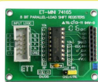
This is 8BIT SHIFT REGISTER PARALLEL-TO-SERIAL DATA CONVERSION that is PARALLEL-IN,SERIAL-OUT for SPI Interface. It receives incoming data as parallel type and it sends out data through OUTPUT as serial type. It supports the maximum CLOCK Frequency at 35 MHz. This board uses IC No.74LS165. Pin DATA IN is 10 PIN BLOCK Type; and PIN OUTPUT is 8PIN HEADER MALE and FEMALE.
