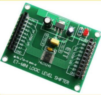
It is Board circuit to connect signal Logic between 5V components and 3.3 V (or 3V) components and uses IC 74CX245 to be medium of connection. Moreover, there is circuit REGULATOR 3.3V on Board.
