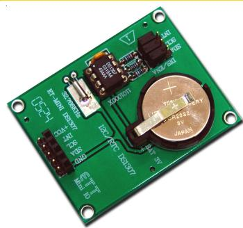
It is experiment of I<sup>2</sup>C BUS as RTC Circuit No. DS1307 size 8 PIN with Battery 3V for backup data in Port RTC, PORT INPUT 5 PIN MALE and FEMALE.
