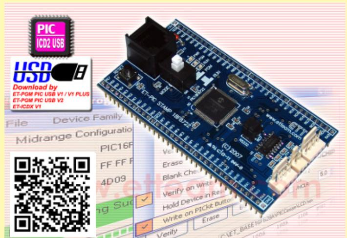
PIC Board of MICROCHIP is designed as compact board that is easy to use or connect with PROJECT BOARD. Moreover, there's necessary devices to use or develop board with [ET-PGM PIC USB V1/V1 PLUS/V2](#), [ET-ICDX V1](#), [ET-PGM PIC PK3/PK3 PLUS](#) that can be connected PORT USB of computer and Board ET-PIC STAMP through standard Connector RJ-11 (ICD2).
