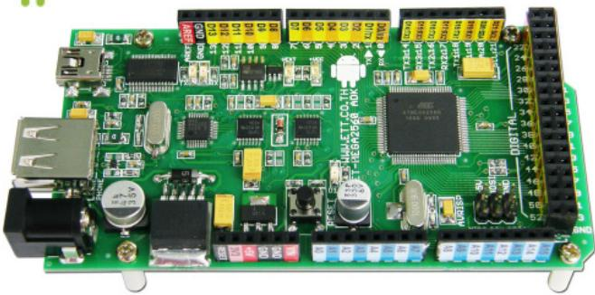
... Nowadays, ETT has developed and used AVR MCU No. ATMEGA2560 and MAX3421 to be Board Arduino that has USB HOST; it supports the connection with USB DEVICE and Android OS devices. It designs and chooses PIN I/O, including board size according to the standard of Board Arduino MEGA.
