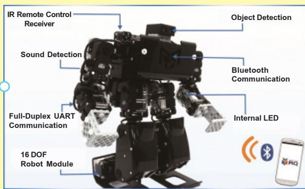
**SENSOR OBJECT DETECTION:** To detect Remote Signal or white object
