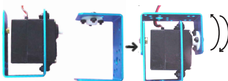
*An example of connecting between R-JOINT SERVO and SERVO MOTOR.
