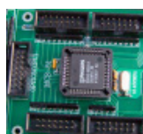
CPU MCS-51 OF ET-LAB3A AS NO. P89V51RD2 WITH 64 KBYTE INTERNAL FLASH MEMORY
