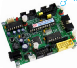
Board Microcontroller version "ET-BASE AVR EASY328 TRAINING BOX", "ET-BASE AVR EASY168 TRAINING BOX", "ET-BASE AVR EASY88 TRAINING BOX", it has the same board's figure but MCU of each version is different.
